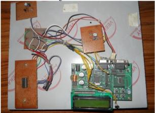
Fig.3. Microcontroller Base Kit
